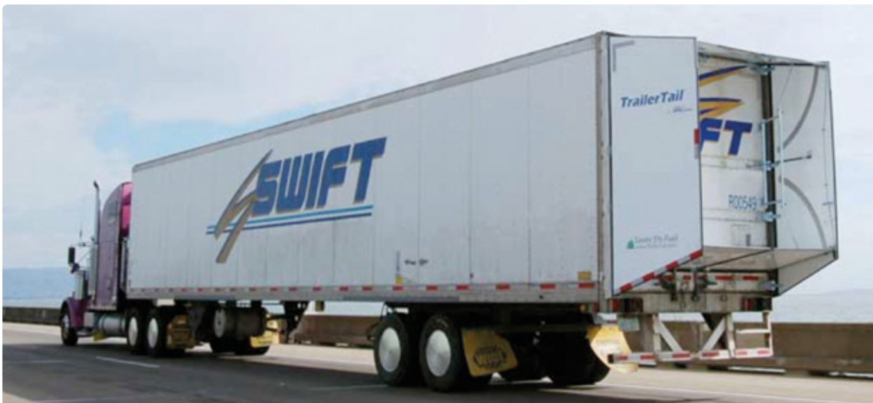
Figure 6 Aerodynamic “boat tail” used to reduce aerodynamic drag
