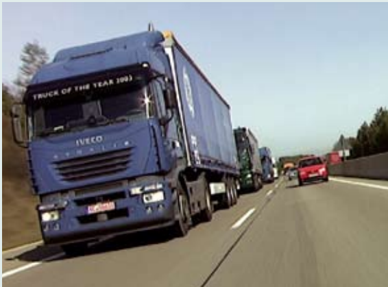
FIGURE 17: ELECTRONICALLY COUPLED TRUCKS ON A GERMAN MOTORWAY WITHIN THE PROJECT KONVOI
